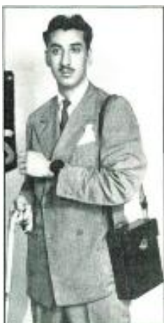
On the eve of his first convention in 1936, Trout demonstrates CBS's new "walking transmitter." The watch is a microphone, the binocular case holds an amplifier and modulator, and the cane serves as an antenna and frequency modulator. Batteries are housed in a money belt.
